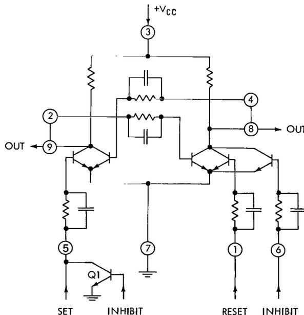
Figure 4—SN514 solid circuit used as a flip-flop.
