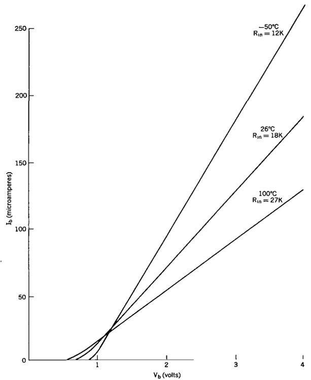
Figure 6—Input resistance of the SN512 solid circuit.
