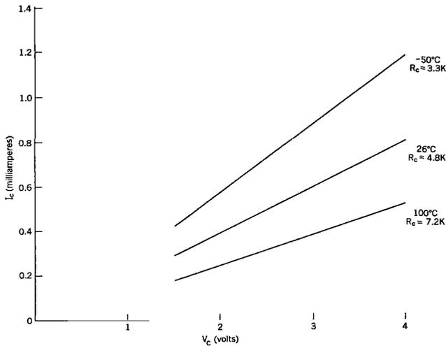
Figure 5—Collector resistance of the SN512 solid circuit.
